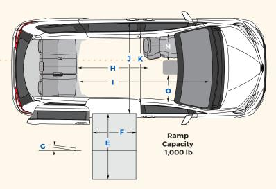
Seats up to seven passengers with an option for three wheelchairs. Seating options may vary depending on available payload.
